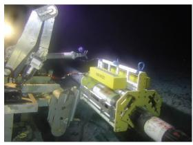
ROV-iT corrosion mapping subsea
